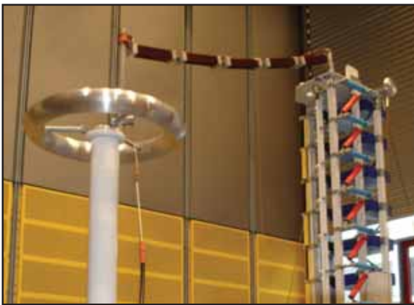
ERITECH Isolated Downconductor being tested
